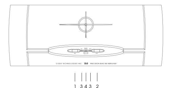
**Note:** If a power interruption occurs to the system the amplifier will power on with the bias off. Press the bias button to resume use of the amplifier.
